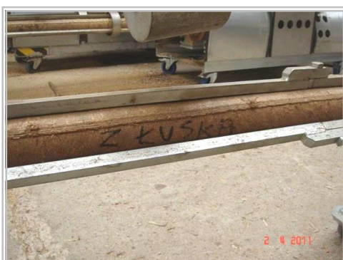
Briquette from Tanzanian grass mixed with rice husks
