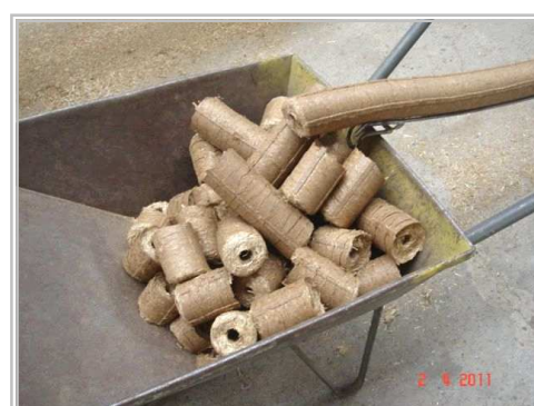
Briquette from Tanzanian grass mixed with rice husks
