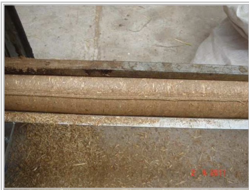
Tanzanian grass briquette inside rod guide
